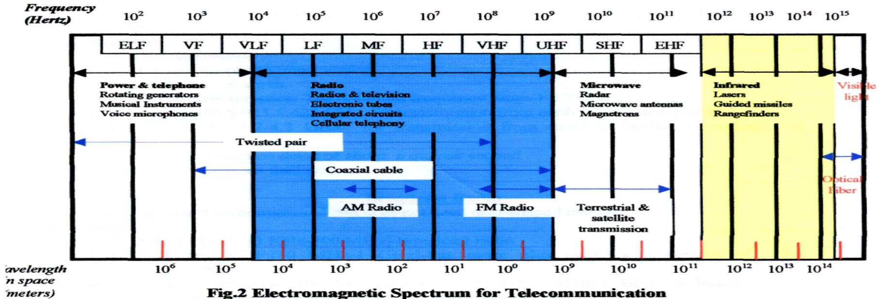
**Fig.2 Electromagnetic Spectrum for Telecommunication**
