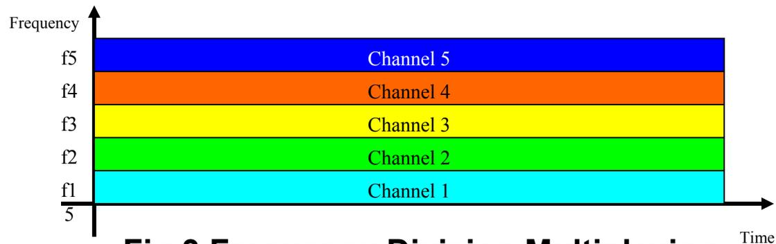
**Fig.3 Frequency Division Multiplexing**
